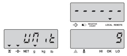
Then press **ENTER** key for determination and enter into calibration mode. **Note**: The weighing unit for local platform is g or lb, while the unit for remote platform is kg or lb.
