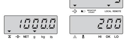
Press TOTAL key to enter into accumulation status mode. At this moment, total accumulated weight is shown in WEIGHT window, total accumulation times is shown in UNIT WEIGHT window and COUNT window displays accumulated count.
