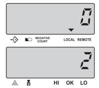
● Press MOVE key to revolve the system-preset zero tracking range. The larger number selected, the wider range (0=off, 1=0.5d, 2=1d, 3=2d, 4=3d).
