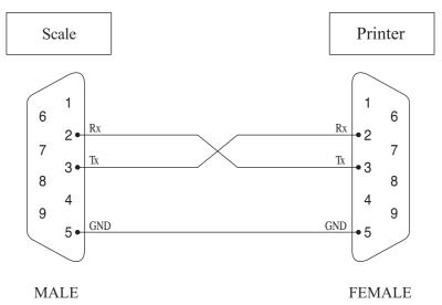
Connect EC-II and Printer using same cable. [male(EC-II) – female(DLP-50)]
