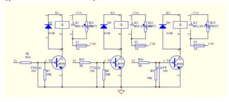
When it is connected with 3 color Annunciator, please use a cable to parallel C1A, C2A and C3A.
