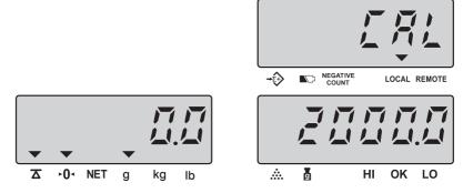
Put a weight on the pan same as what exactly shown in the UNIT WEIGHT window, then press the ENTER key to confirm the operation.
