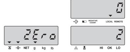
● Press **MOVE** key to revolve the system-preset zero display range (0=off, 1=0.5d, 2=1d, 3=2d, 4=3d).
