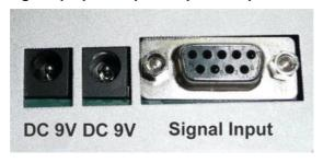
Use our standard cable to connect the signal input port with the scale or other equipment. And these two ports for power adaptor must be connected to make sure the control box is workable
